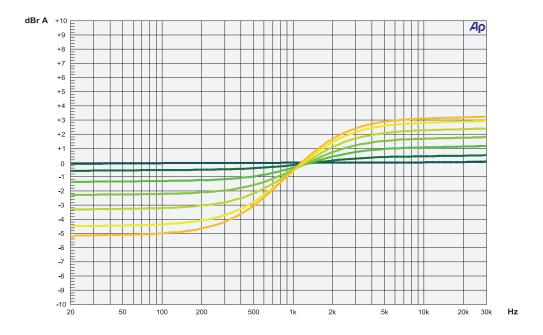
This diagram shows a variation of center frequencies with the EQ gain controller turned fully clockwise (HI). The x10 button shifts the complete frequency area by a factor of 10. With settings in the border areas of the covered frequencies it is also possible to realize 'almost' shelving filters, but in these cases the level has to be adapted with the gain controllers.
