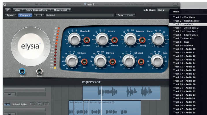
The Mpressor also has a sidechain function so you can trigger it from any other track, input or buss in your DAW. Very useful especially considering all the weird and wonderful shaping possibilities it already gives you
